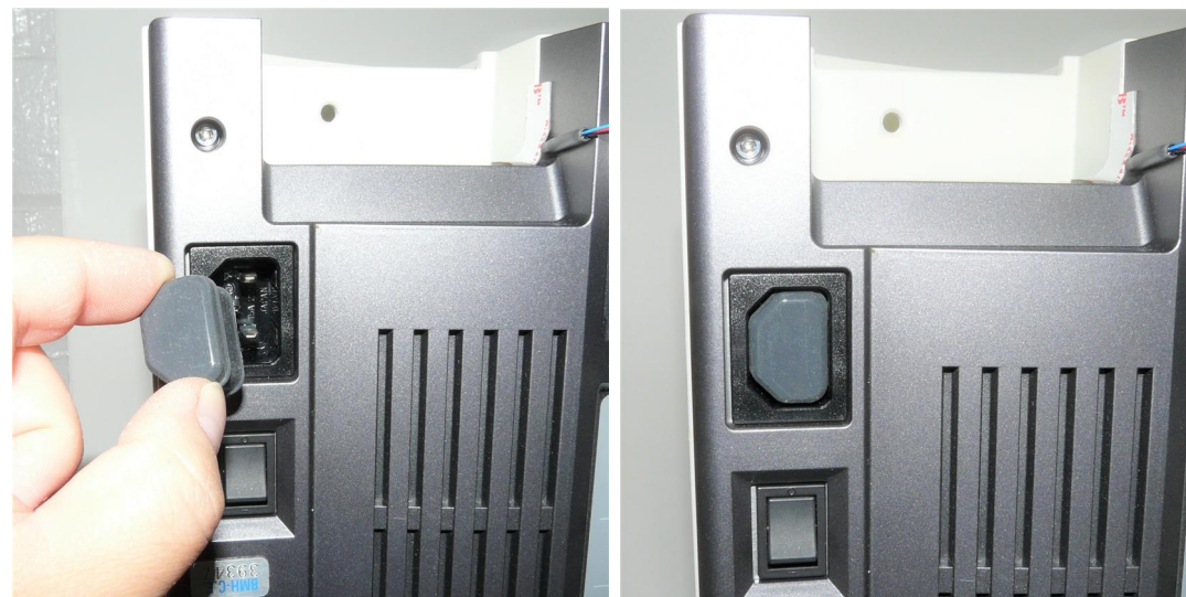
(2) Install PN 10736 rubber blocking plug in the now-obsolete AC receptacle as shown in the photos.
