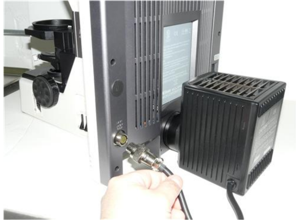
(1) Be sure the AC power is unplugged. Disconnect the original lamp power cable.
