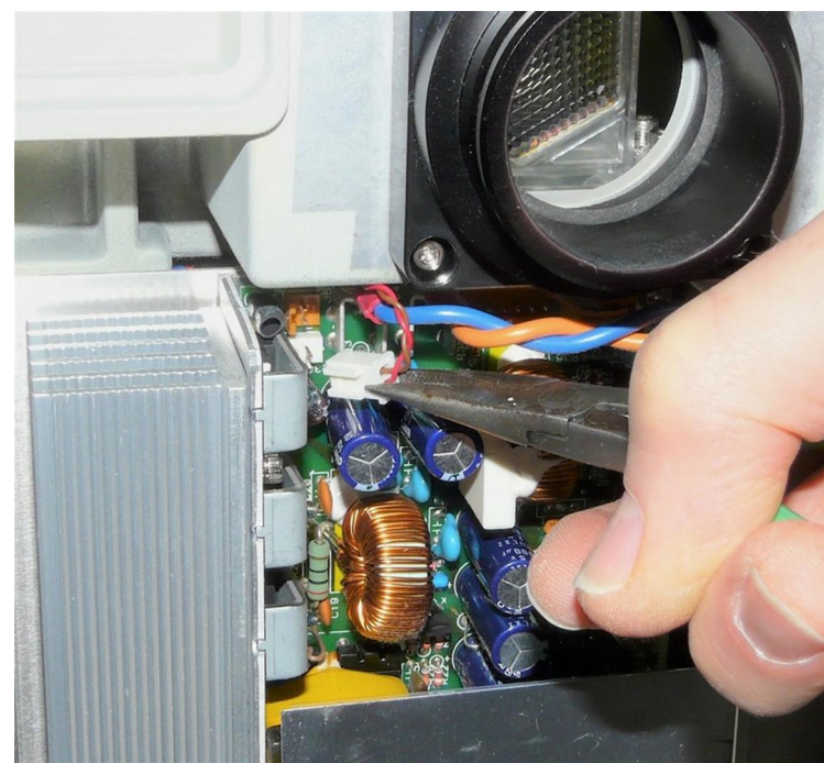
(4) Disconnect the red and brown cable with the white plug from the power supply.
