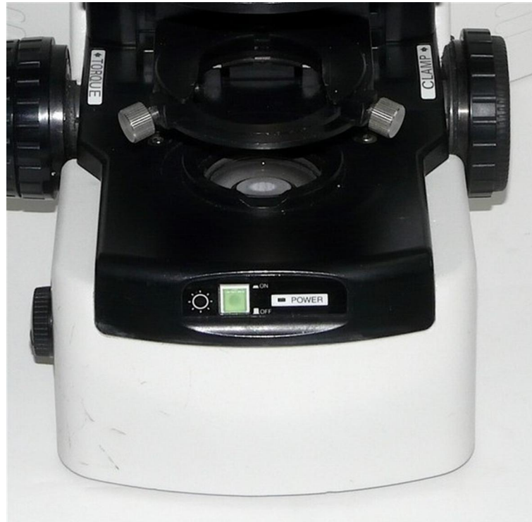
(1) The control on the front of the microscope will be obsolete. Intensity control for the new illuminator will only use the knob on the left.
