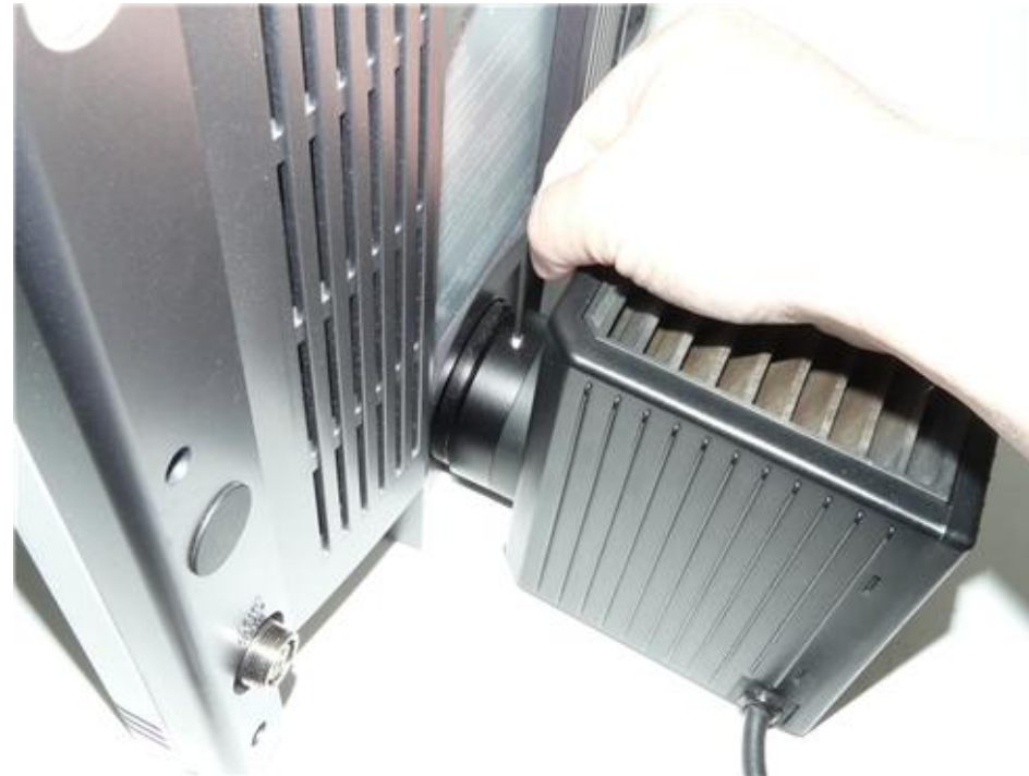
(2) Loosen the set screw holding the original lamp.
