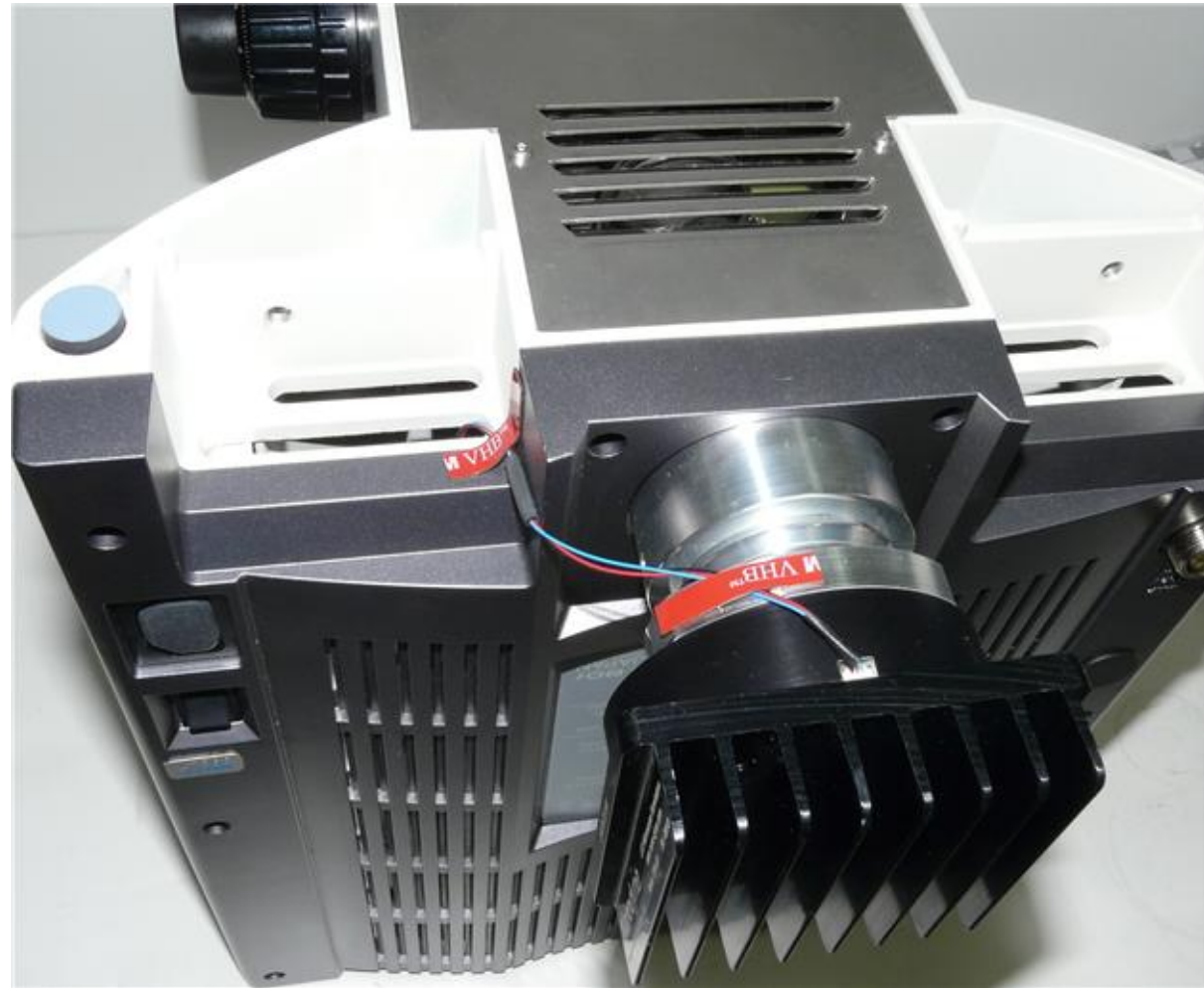
(1) Secure the pot cable with the 3M VHB tape (red, in above photo). Secure it inside the microscope also, where the cable goes by the focusing gear.
