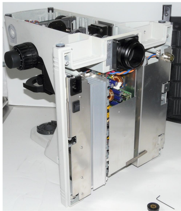
(3) Remove the back cover. It is held by 8 socket head screws. Use a hex key to remove them.
