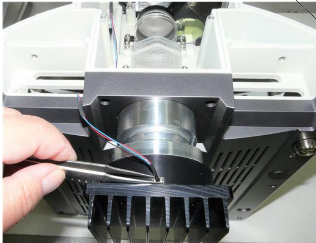
(4) Connect the pot cable to the illuminator.
