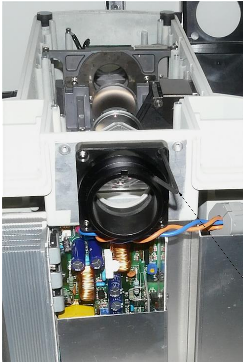
(1) Do not remove the original illuminator mount. Nanodyne adapter will fit as is.
